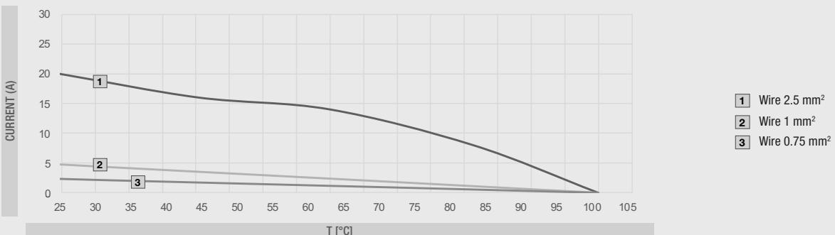
**N.B.:** for the TH387U range there are two graphs referring to the derating curve, as the 3Poli version supports up to 2.5mm<sup>2</sup>, while the 4Poli version supports the 1.5mm<sup>2</sup> version.
